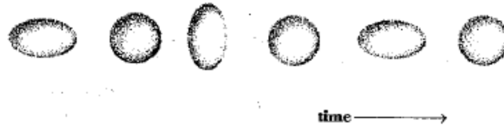
FIGURE 24.11 The oscillations of a liquid drop.
